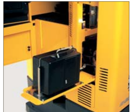
Easily accessible aggregates through foldable doors
